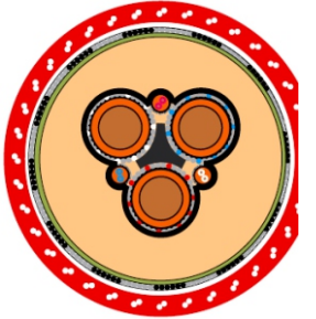
10-core conductor BiTflex O2nGcekż/w-GW
